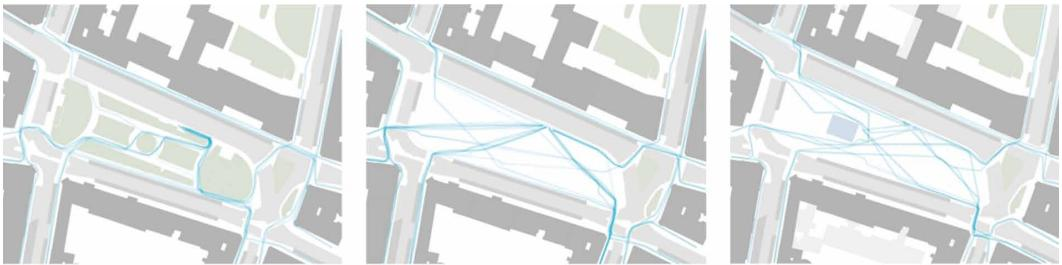
Figure 8. 3D modelling of Aumannplatz and its surroundings with integrated water playground and simulation of pedestrian flows to and from defined points of interest. Own illustration (© AIT)
